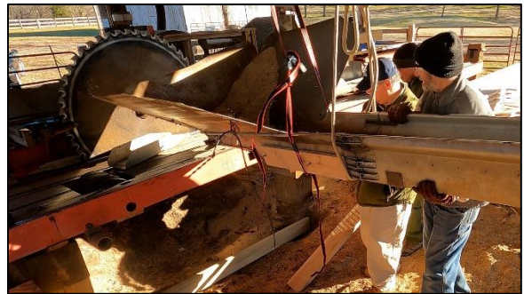
Sawdust elevator being put back in the hole!
