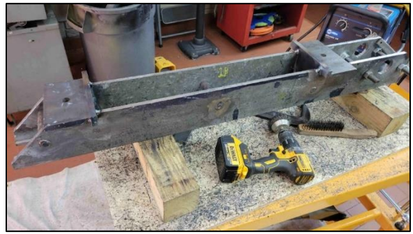
New headblocks almost ready to install
