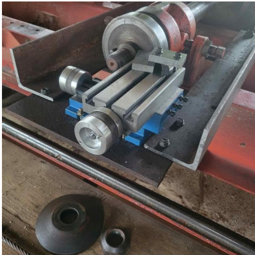
Custom jig for machining the mandrel collar
