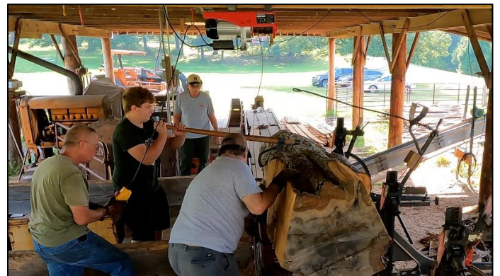
Matt and Cody rolling a big log with the new log rolling winch and a cant hook
