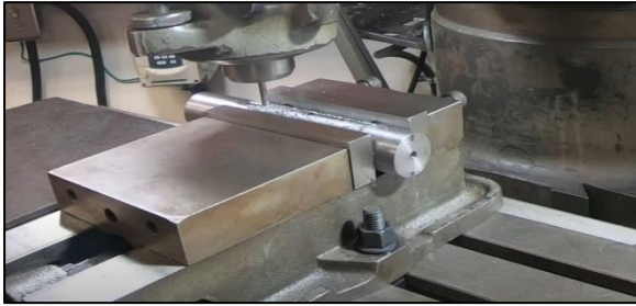
New pulley pin being machined.
