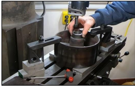
New bushings being test fit.
