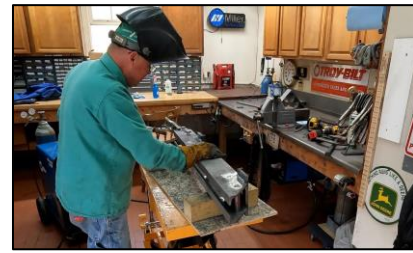
New head blocks being welded.
